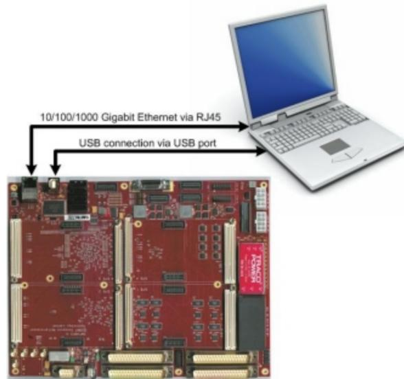
The board support package includes a complete web server application running on the [PowerPC™ 405](#) to demonstrate the SMT6058 TCP/IP API and functionalities.
