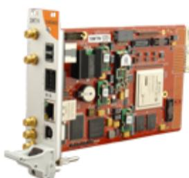
is a **rugged and scalable** solution that can be mounted into a strong 3U PXI chassis/ enclosure. The Series-1 is dedicated for embedded applications in which several SMT100s can be **stacked together** and be used in standalone mode or in combination with a single board computer.
