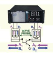
VTD have successfully launched <u>SWAP-</u> X402: an advanced instrument for the time domain load-pull characterization of microwave transistors (see: <u>introduction to</u> <u>measurements for power transistor</u> <u>characterization</u>). **SWAP-X402** measures the time domain waveforms of voltages and currents at the transistor terminals under realistic operating conditions. The additional time domain data result in an
