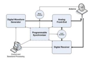
**Software defined radar** (SDR) platforms can adaptively switch between different modes of operation by modifying both transmit waveforms and receive signal-processing tasks in real time. Key components of such architectures are high-speed A/D and D/A modules along with FPGA devices and fast digital signal processors allow for maximum flexibility in algorithm design. The <u>ElectroScience</u>
