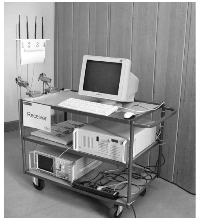
Fig. 1. 4-Antenna Receiver of the STARS2 Test-bed Mounted on a Trolley.
