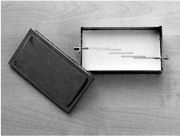
Fig. 8. Photo of BPF Designed in Micro-Strip Technology.
