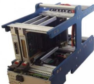
The [VT330](#) VPX-Test Platform is a 3U OpenVPX rack with a 3-slot backplane, power supply and fan. The open frame design of the rack makes it ideally suited for software, firmware and hardware development of 3U VPX modules. The 3-slot backplane has one payload slot and two peripheral slots with Fat Pipe (FP) connections between the payload slot.
