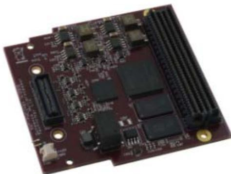
This, the [SMT-FMC211](#), with own on-module FPGA, will provide four channels of 16-bit Digital to Analog @ 1.2GHz when combined with a VF360
