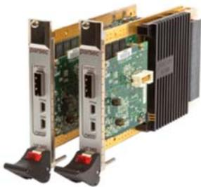
The [VF360](#) is a 3U OpenVPX module that leverages the Altera Stratix® V FPGA and Texas Instrument's Keystone® Multicore DSP technology to provide a ultra-high performance processing platform in either air-cooled or conductive configuration. Extra I/O expansions with our [VITA57.1 FMC-HPC](#) Modules.
