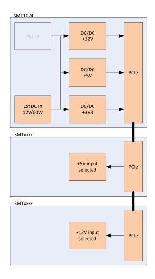
This system shows the use of  $2 \times SMT1024$  each supplied from a PoE source. The 1st SMT1024 provides +12V and +3V3 (low power requirement), and the 2nd provides the +5V rail. Again, the SMT6678s use different power rails.
