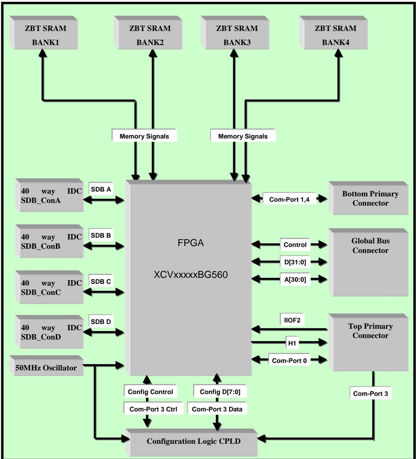
Figure 1: SMT358 Block diagram
