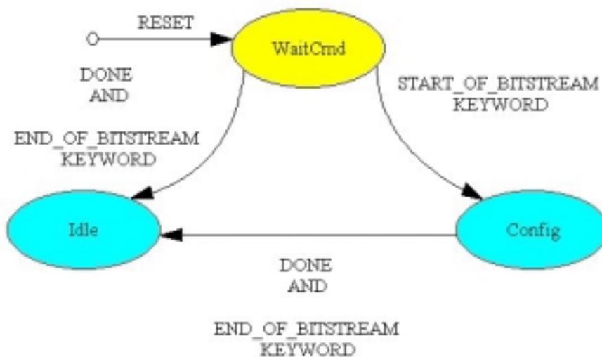
**Figure 8: FPGA reconfiguration**
