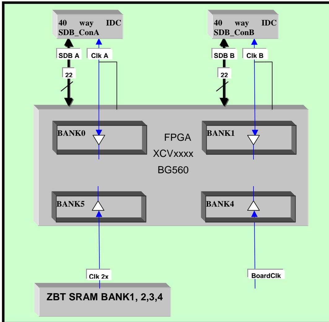
Figure 6: Global Clock Buffers assignments in the Virtex/E
