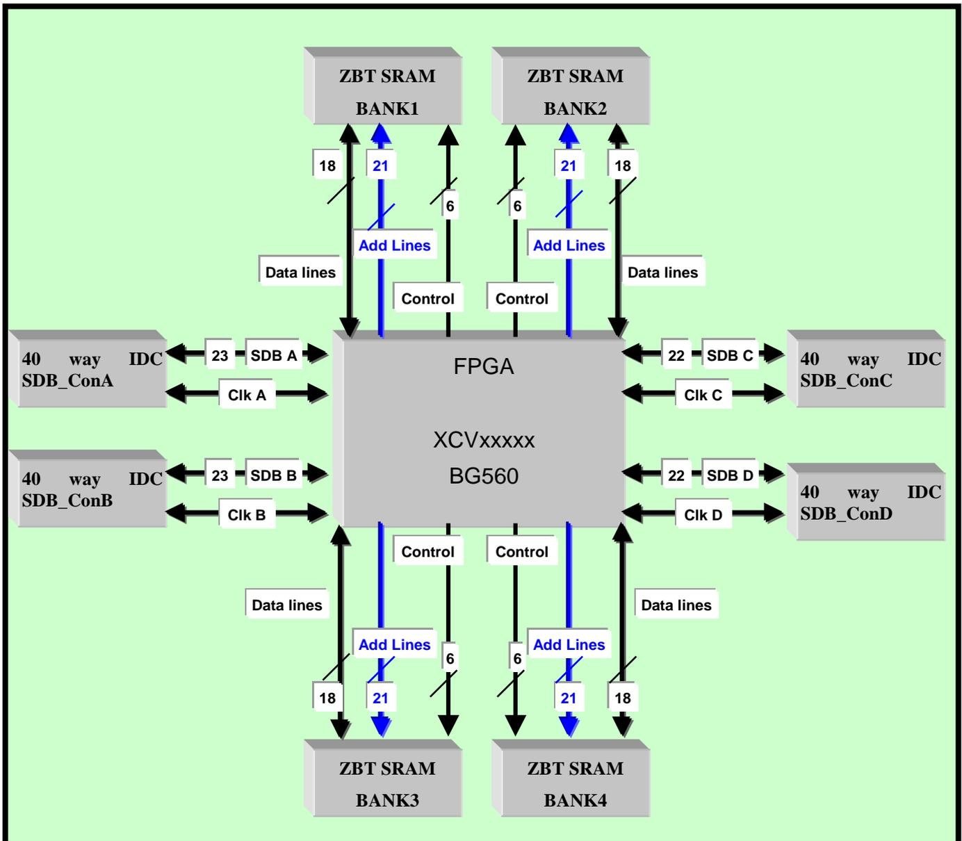
Figure 3: FPGA, Memory and SDB Communication Channels
