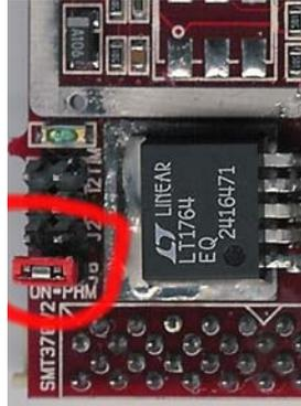
When J8 is not fitted, the user can reprogram directly the FPGA.
