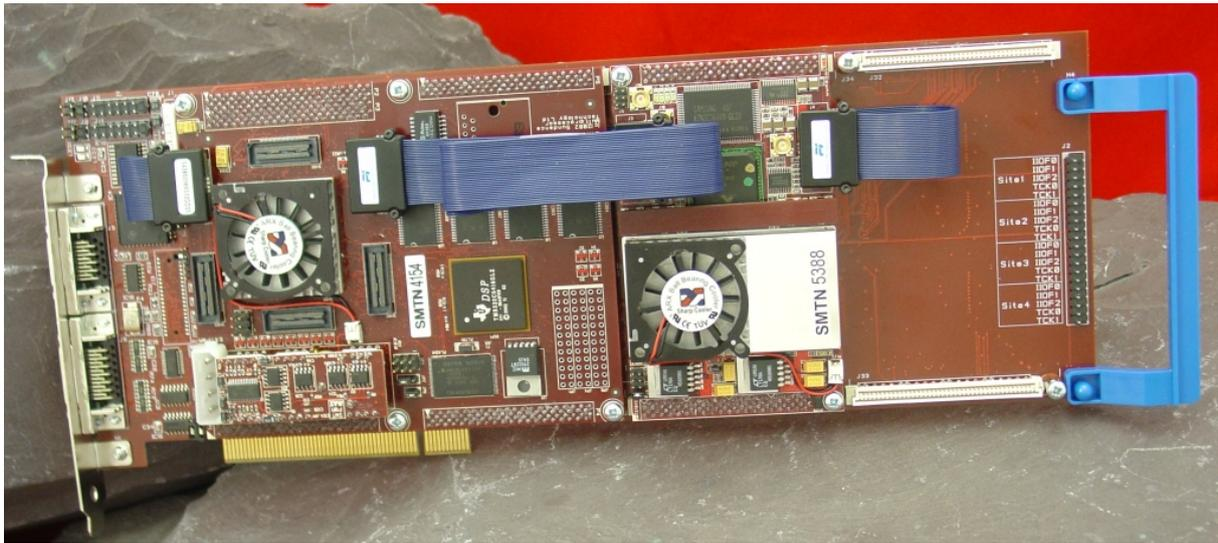
The following picture shows the CommPort connection at the back of the SMT310Q. Note that the FMS are 'twisted', i.e. one end should be blue and the other should show silver pins.
