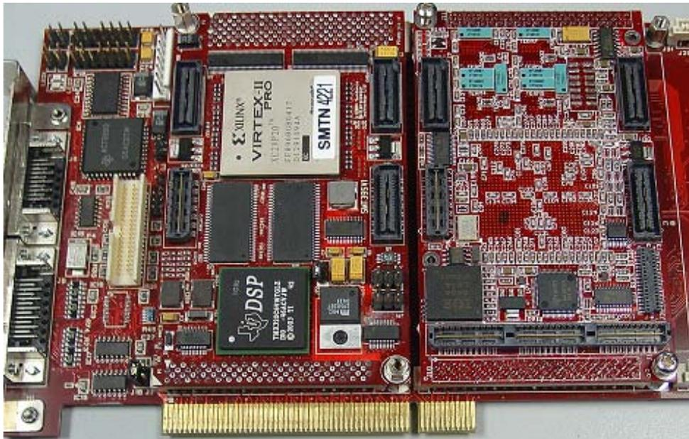
d – Place the SMT391 on top of the SMT338-VP. Make sure that both modules fit firmly.
