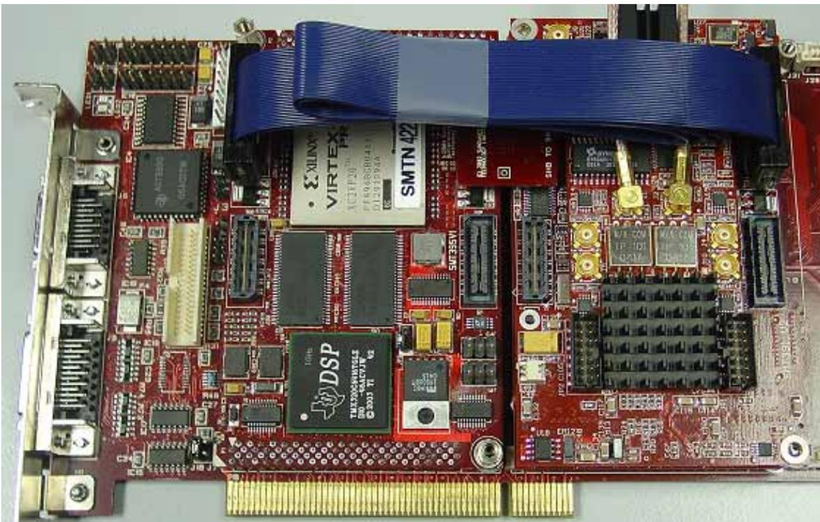
The following picture shows the Comport connection at the back of the SMT310Q. Note that the FMS are 'twisted', i.e. one end should be blue and the other should show silver pins.
