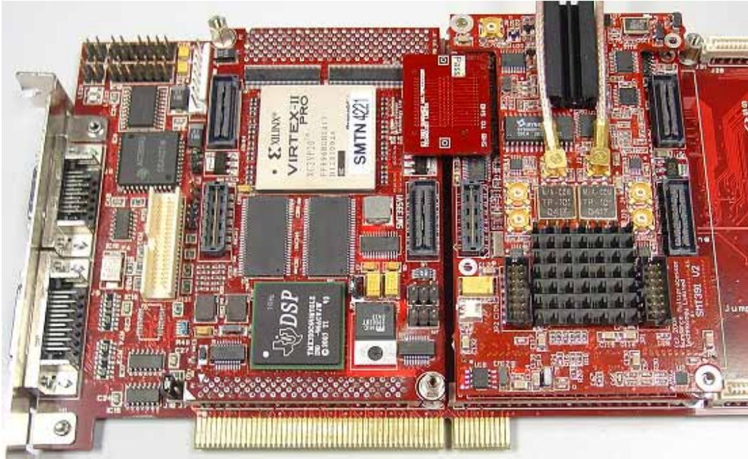
6 – Connect external sources to J1 noted G (ChQ), J2 noted C (ChI) via MMCX-BNC cables. Make sure that the external signal meets the input characteristics of the *SMT391-VP* described in the *SMT391-VP User Manual*.
