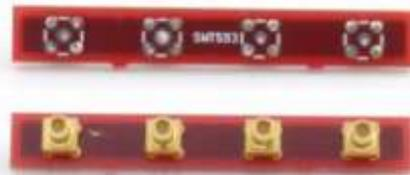
Figure 19 - SMT593 Loopback pcb.
