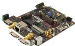
The [OI110](#) is a PC/104 COTS board that leverages a Dual-Core ARM9 + Xilinx Kintex-7 FPGA (Zynq SoC) and a Dual CameraLink, running at up to 85MHz, interface with Dual SATA-3 ports and PCI Express expansion via the PCIe/104 OneBank stackable connector concept.
