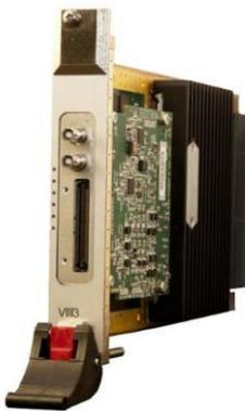
The [VI113](#) is a 3U OpenVPX COTS board that leverages on an Altera Stratix-V FPGA, coupled with a Texas Instruments Keystone® Multicore DSP and Dual SDI Video Input/output interfaces and a number analog and digital interfaces to provide a video processing stand-alone system. The VI113 can either be supplied in conductive cooled or air-cooled variations for integration into bespoke OpenVPX enclosures.
