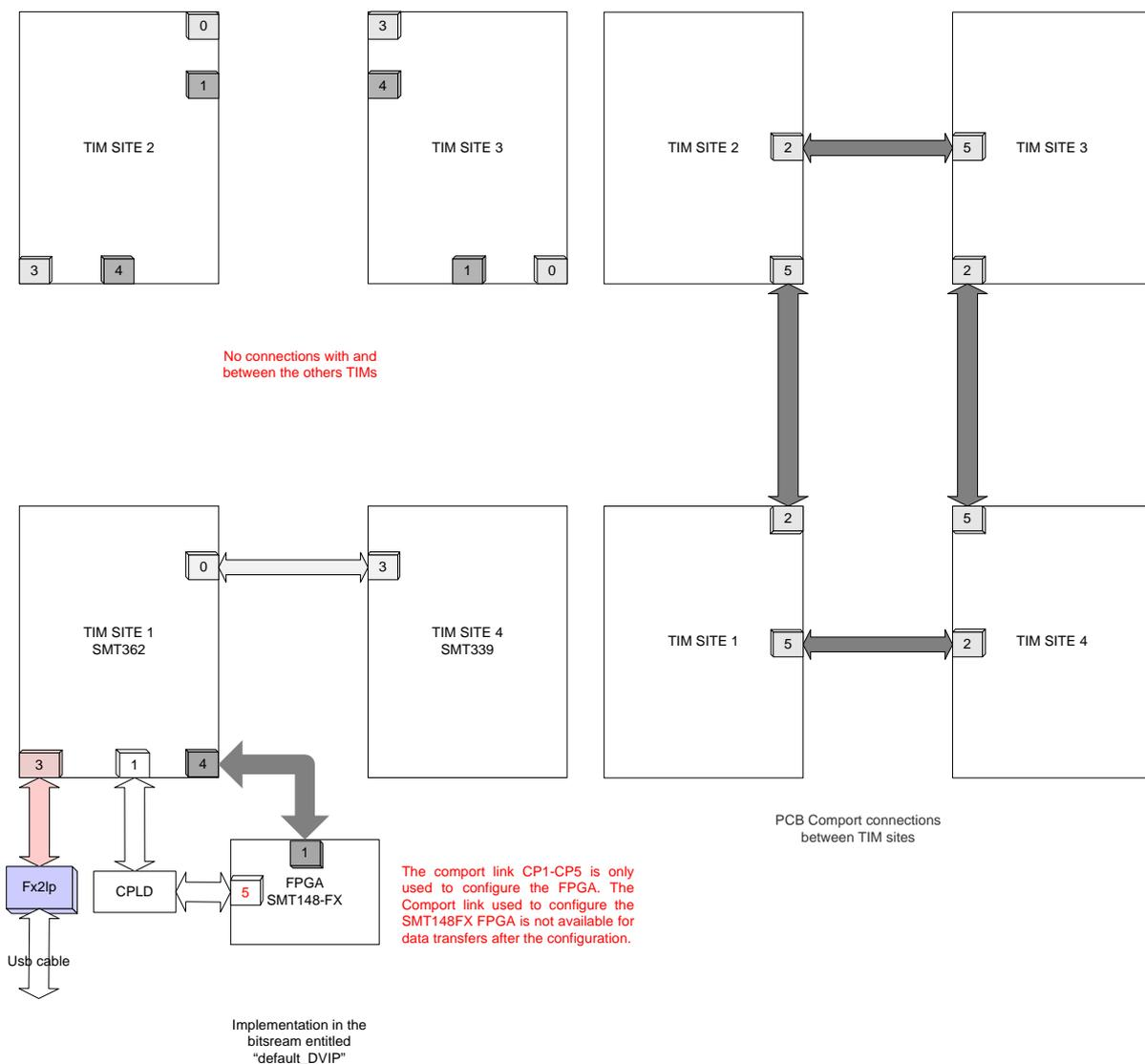
**Figure 9 : DVIP bitstream comport configuration**
