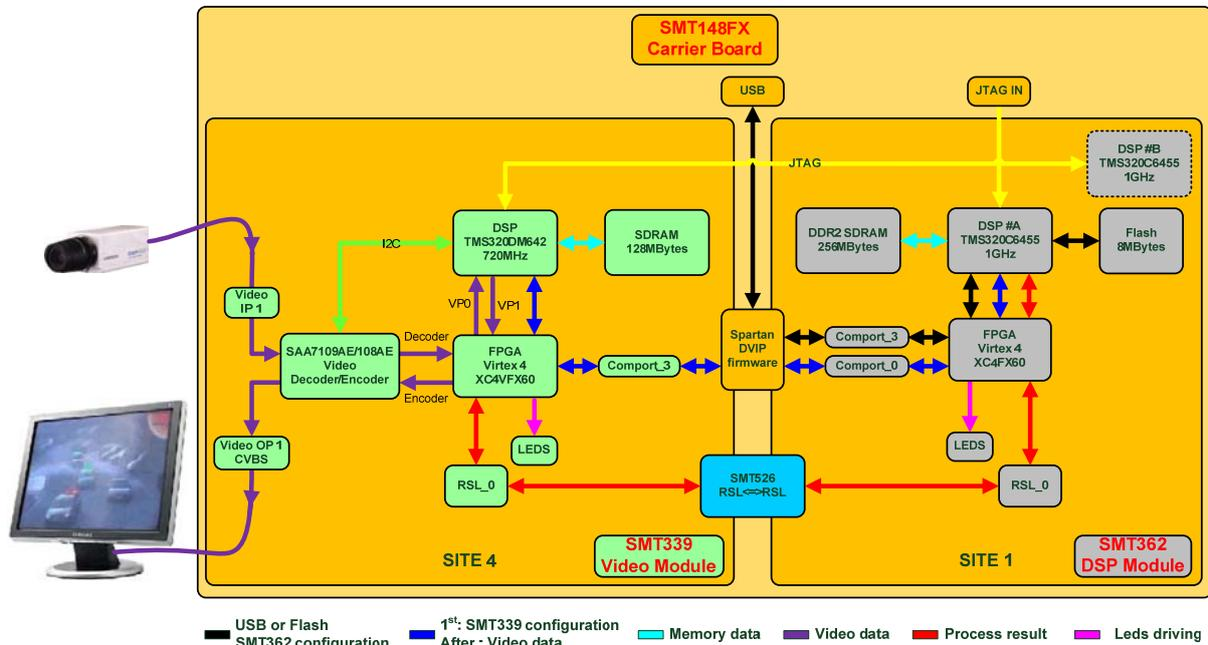
**Figure 10: RSL application diagram**
