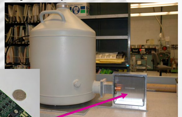
Figure 7: XH cryostat at LBNL
