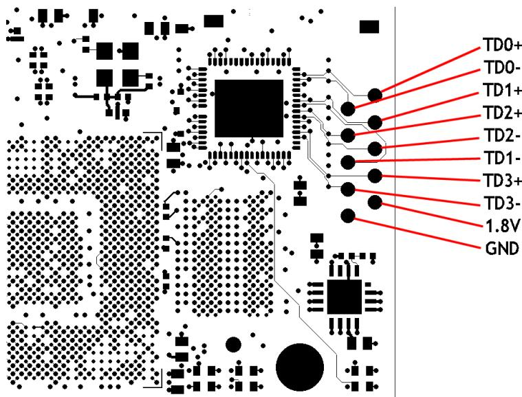
There are three EMAC interfaces to the FPGA which requires 39 I/O pins, and a further 2 for the MDC/MDCIO interface.
