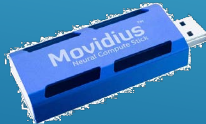
Movidius Neural Compute Stick Interface: USB3.0
