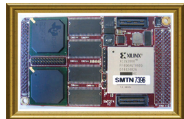
The SMT374 dual floating point DSPs and Virtex-II FPGA
