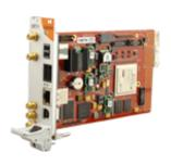
Two major product families have been released in Year 2009: Series-7 (SMT700) and Series-1 (SMT100), respectively 3U PXI Express and PCI/104-Express form factors. Both hardware solutions feature a range of Virtex-5 LXT, SXT and FXT FPGA devices which implement a PCI Express interface (x4 lanes at 2.5Gbps), which is essential for high-bandwidth applications. The SMT700
