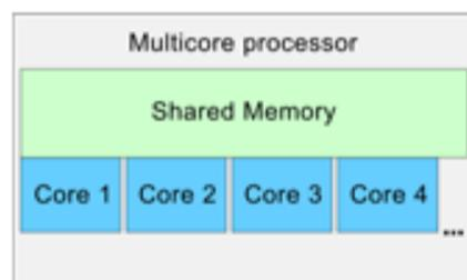
**Multicore systems** are defined as single-chip computers containing two or more processing cores each connected to a common shared memory. These devices and multicore-based architectures are announced as the ultimate solution to the performance problems faced by embedded systems. However, design engineers may feel reluctant to jump into this new technology since at this early stage the lack of efficient software programming
