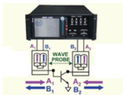
VTD have successfully launched [SWAP-X402](#): an advanced instrument for the time domain load-pull characterization of microwave transistors (see: [introduction to measurements for power transistor characterization](#)). [SWAP-X402](#) measures the time domain waveforms of voltages and currents at the transistor terminals under realistic operating conditions. The additional time domain data result in an
