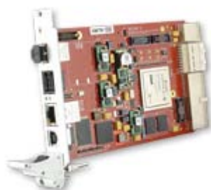
SMT700: 3U PXI Express (Industrial-grade Fibre solution)
