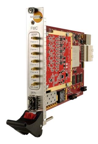
PXIe FPGA + Multi ADC FMC Integration
