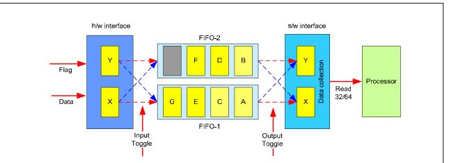
When the processor makes a 32-bit read access, the software interface will take a single 32-bit word from the FIFOs, and change the state of the "Output toggle" signal. In the case of a 64-bit read operation, the software interface takes two 32-bit words from the FIFO and leaves the state of the "Output toggle" unchanged.
