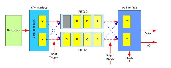
The software's X and Y registers are connected to the two FIFOs by a switch that can toggle between connecting X to FIFO-1 and Y to FIFO-2 and connecting X to FIFO-2 and Y to FIFO-1.
