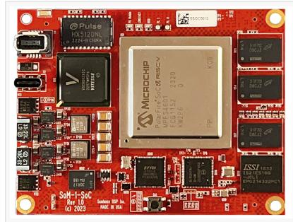
The SoM1-SoC includes a Microchip PolarFire FPGA
