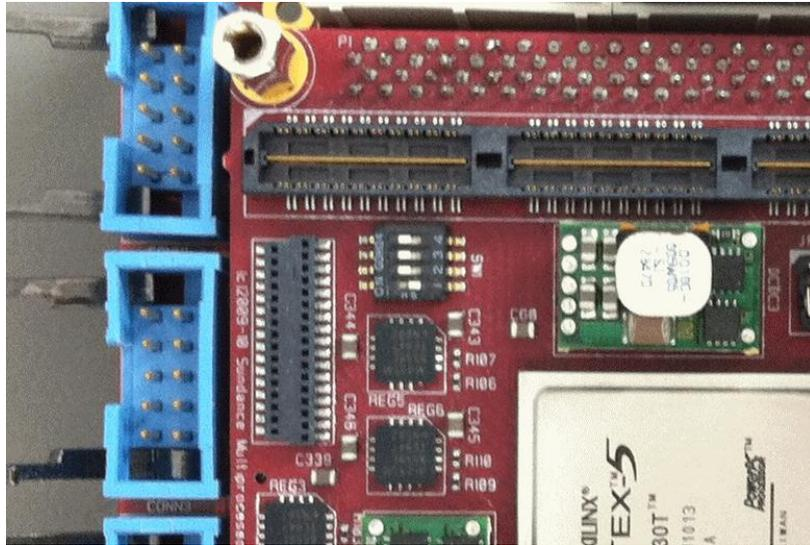
Build the system with the SMT372T screwed onto the SMT111 (this creates an EVP6472). Using two SLB extenders (with JTAG breakout), attach the SMT946 to the EVP6472.
