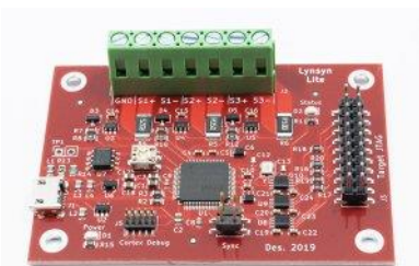
Photocaption 1: Lynsyn Lite – a low-cost power measurement tool for the development of energy-efficient embedded and CLEC systems
