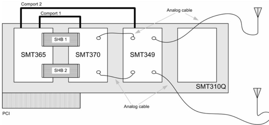
Figure 2. Block diagram of WHERE platform
