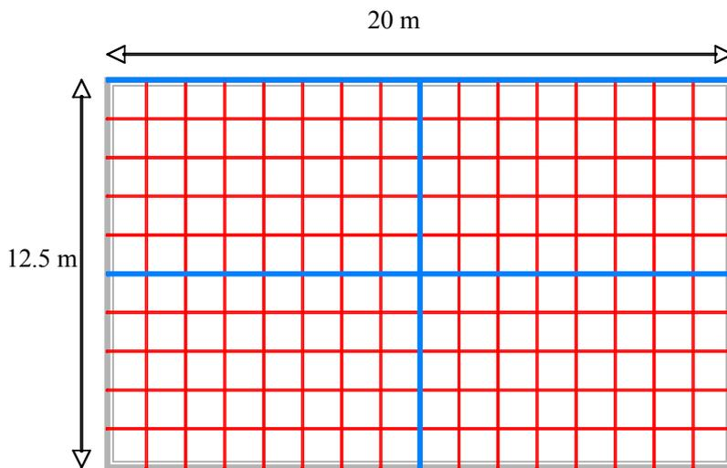
Figure 3. Measurement grid where transmitter positions are shown in blue and receiver positions are in red.
