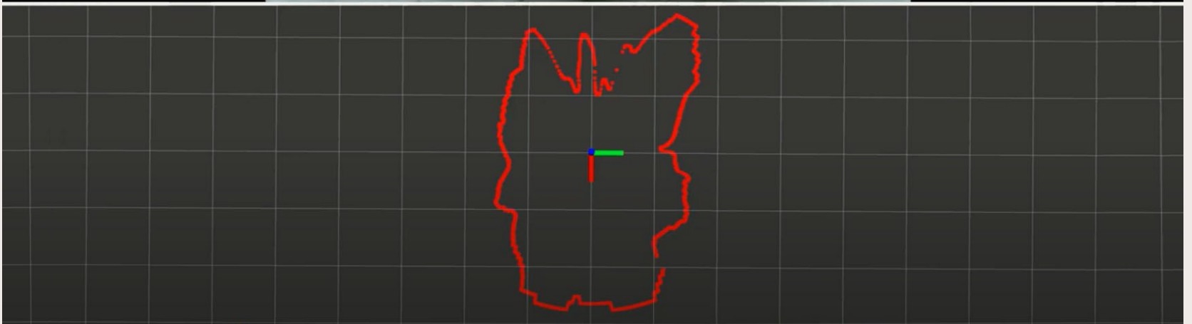
Simulated 2D laser scan output overlaid on 360° RGB with real-time 360° mapping output in ROS
