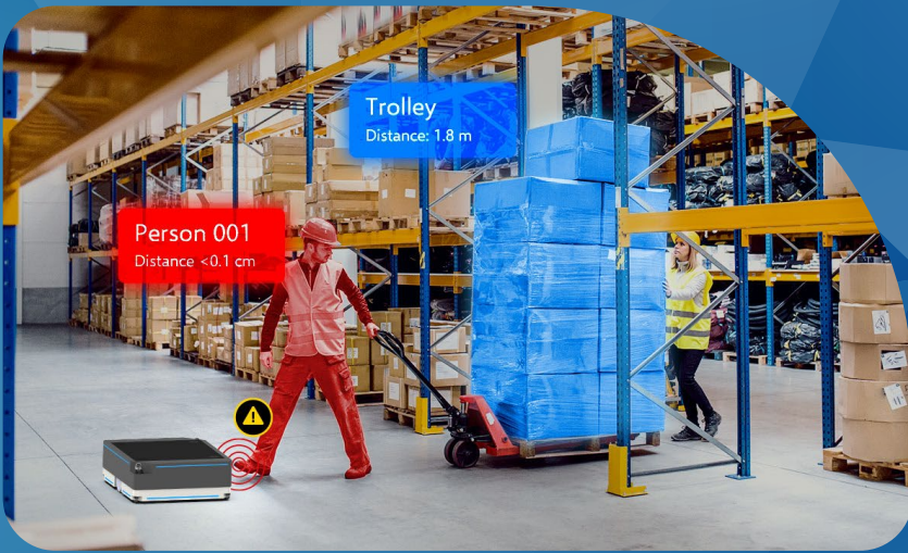
Ultra-wide field of view visual obstacle detection in a warehouse detecting pallet stacks and humans from head to toe
