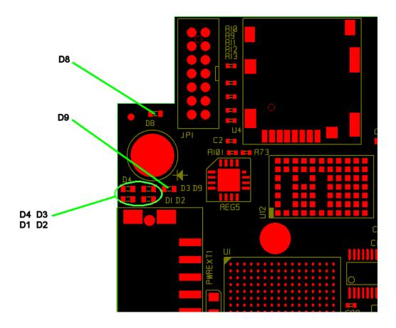
LEDs D1 to D4 are connected directly to the FPGA using pins H20, H19, H13 and H14 respectively.
