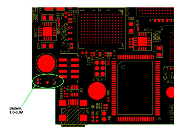
BAT1 is used to supply a 1.0 to 3.6V DC supply. It is only required if bitstream encryption is enabled. The security key is held within the FPGA in a battery backed location.
