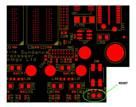
Either pressing SW1 or shorting JP10 will cause an active low reset to the FPGA pin AH17.
