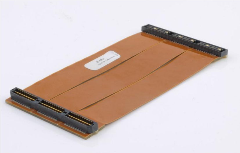
Figure 2 - SLB cable - FlexiPCB.
