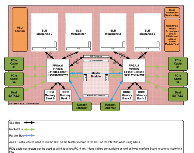
The SMT166 SLB carrier board architecture is shown below:
