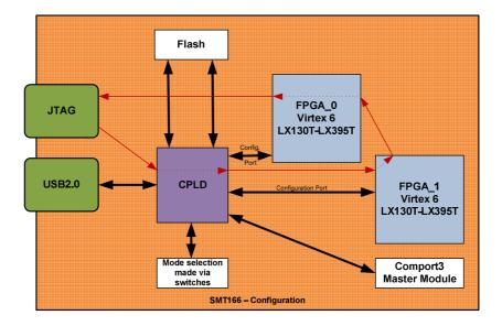
The CPLD contains a configuration that allows the two Virtex 6 FPGAs to be programmed/configured upon reset or power-up. The configuration data is stored in a flash memory device. The flash contents may be programmed using SMT6002.
