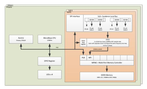
The Virtex 6 FPGA contains the following configuration shown below:
