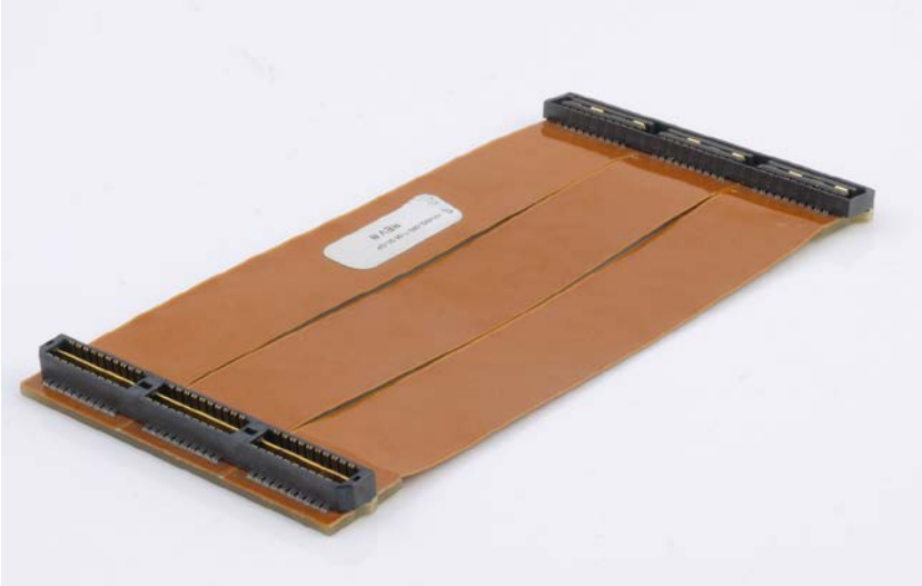
Figure 2 - SLB cable - FlexiPCB.
