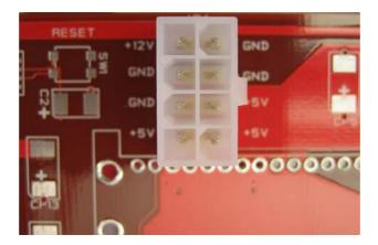
The +12V source is input to a DC-DC converter module, which produces +/-12V to the TIM sites.
