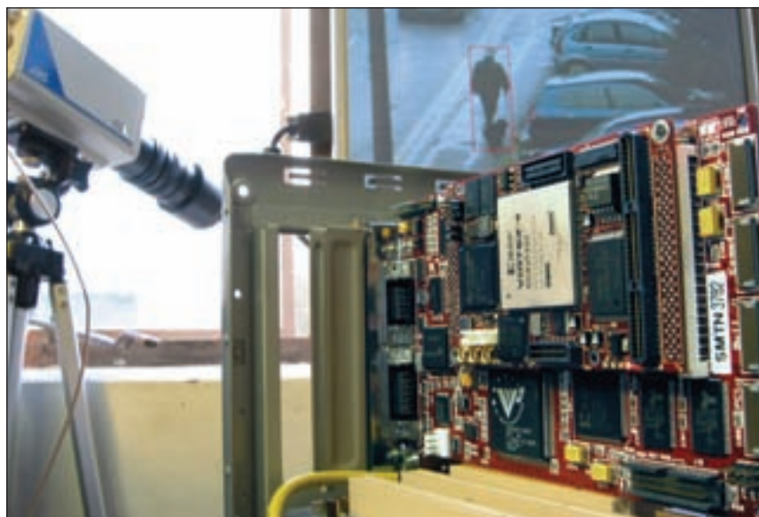
Figure 3 – The Sundance SMT339 in a simple system
