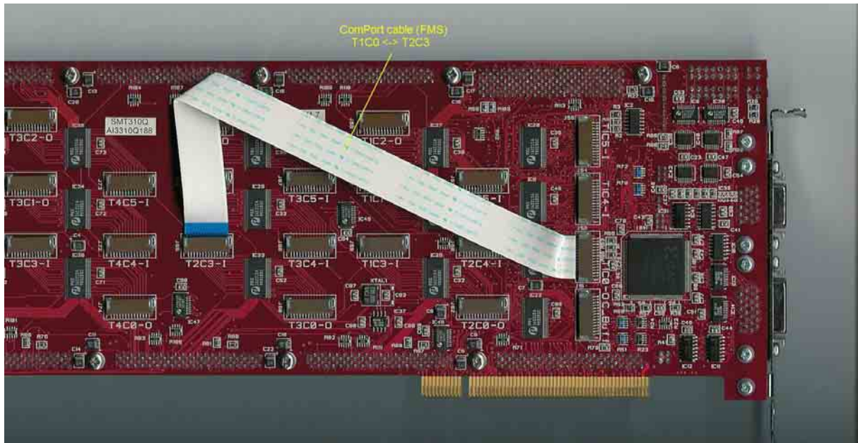
Figure 4 - Example of installation - ComPort connection.
