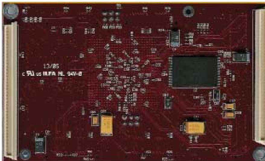
Figure 15 - Main Module (SMT368) Solder Side.
