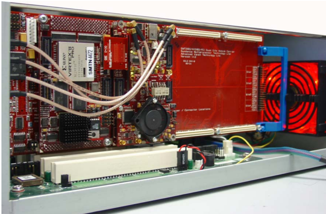
Figure 1 – Fan across PCI.
