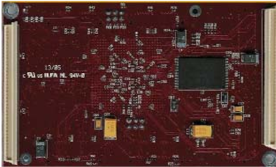
Figure 19 - Main Module (SMT368) Solder Side.
