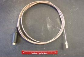
• The output cable is built with two SMB connectors and a S-Video plug
