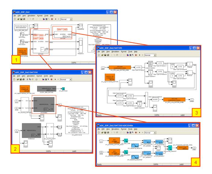
SMT8096 model. *Picture 1* shows the top level containing an SMT350 "block" and an SMT395; interconnections are made with SHB channels; the input stimuli in this case are two analogue sine waves; a few scopes are employed to monitor internal and output signals.
