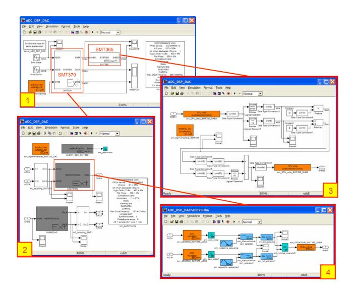
SMT8036 model. *Picture 1* shows the top level containing an SMT370 and an SMT365; connections are made with SHB channels; input stimuli in this case are two analogue sine waves; a few scopes are employed to monitor internal and output signals.
