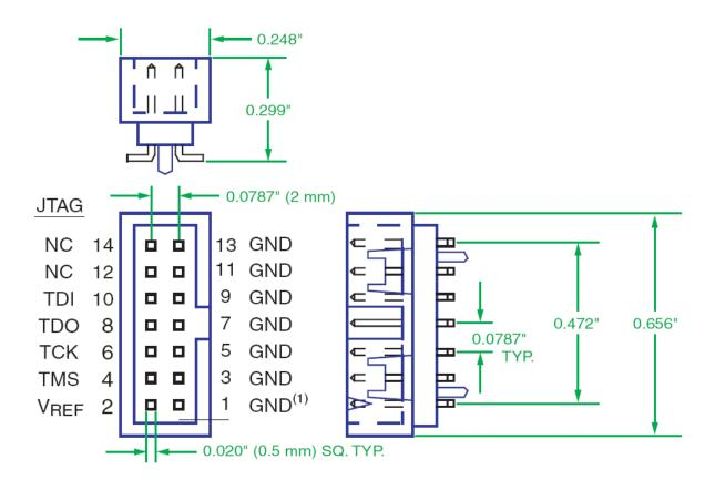
This connector has been chosen because it can connect easily to a Xilinx Parallel IV cable using the ribbon cable provided by Xilinx.
