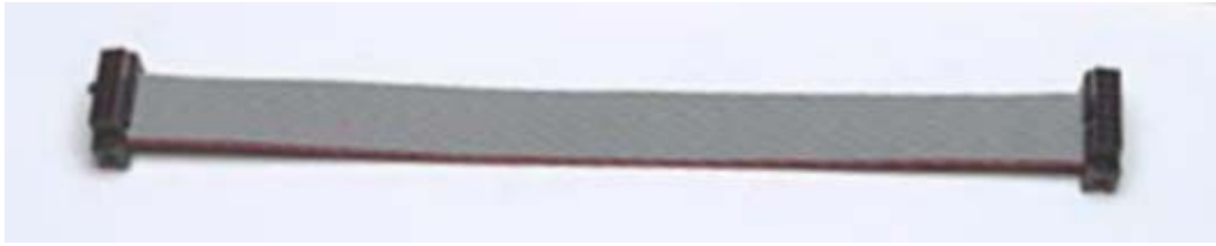
Figure 9 - Photo of a Xilinx Parallel IV cable and its ribbon cable for JTAG connection
