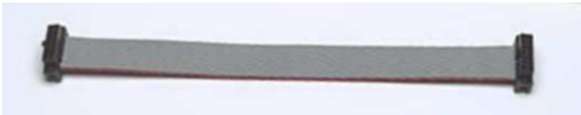
Figure 13 - Photo of a Xilinx Parallel IV cable and its ribbon cable for JTAG connection The JTAG connector should only be needed when reprogramming the CPLD. The FPGA is accessible from the host using the SMT6002 software.
