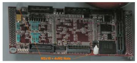
c - Place the SMT338 on the second site (SMT365 already on first site) on the SMT310Q and fit two metal pillars (3.3 Volts).
