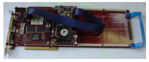
The following picture shows the CommPort connection at the back of the SMT310Q. Note that the FMS are 'twisted', i.e. one end should be blue and the other should show silver pins.
