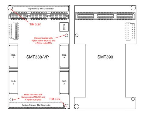
a - First, fit two Nylon screws (M2x10), pointing out (the head of the screws on bottom side).
