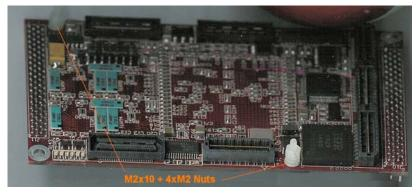
c – Place the SMT338 on the second site (SMt374 already on first site) on the SMT310Q and fit two metal pillars (3.3 Volts).
