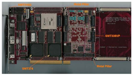
d – Place the SMT390 on top of the SMT338-VP. Make sure that both modules fit firmly.
