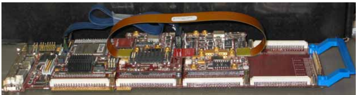
Figure 2: the cable connections of the SMT8101 system
