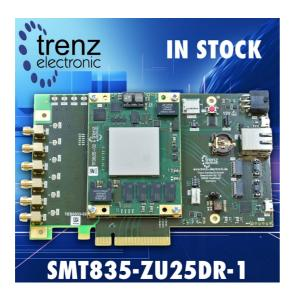
The SMT835-ZU25DR-1 is a PCI express ZynqRF system comprised of the TEB08035 carrier board and the TE0835-02-MXE21-A RFSoC module.
