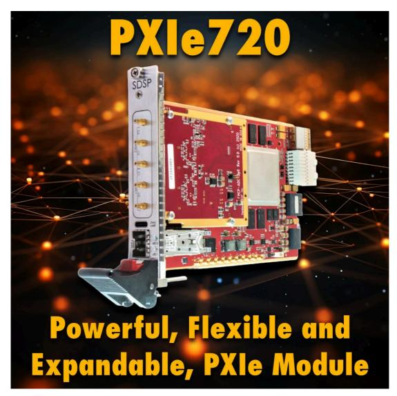
Built around the AMD/Xilinx XCKU060 FPGA, the PXIe720 delivers high-speed data processing with 8GB of DDR4 memory, 10Gb Ethernet, and a PCIe Gen3 x4 interface. Onboard QSPI flash supports multi-boot, while JTAG enables real-time debugging. With an FMC+ site for expansion and White Rabbit precision timing via SFP+ fibre, it's ideal for signal processing, data acquisition, and quantum computing research.
