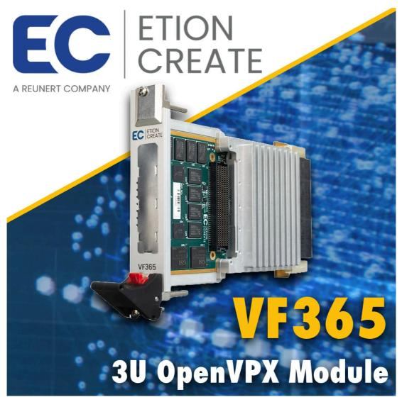
Designed for radar, SIGINT, electronic warfare, software-defined radio, networking, and video applications, the VF365 delivers high-speed data throughput with a VITA 57 FMC site for flexible I/O expansion and 40G Ethernet support, enabling seamless integration. Designed for versatility, it is available in both air and conduction-cooled configurations, ensuring reliable operation across a wide range of demanding applications.
