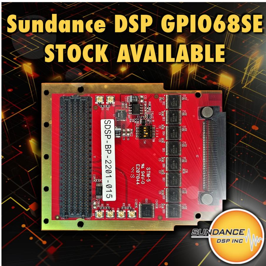
FMC-GPIO-68SE is conduction-cooled HPC FMC. It provides 68 Single-Ended GPIOs through a connector at the front bezel. The IOs are taken through level translator ICs which are auto-sensing and can convert from 1.8V to 3V, or 5V, and vice versa.
