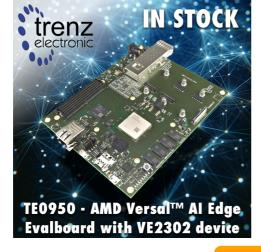
We have three units in stock of the Trenz Electronic, TE0950-03-EGBE21A, with a lead time of 30 weeks for additional units; take this opportunity to get one now. It is an AMD Versal™ AI Edge VE2302 device-equipped SoC evaluation board. It features 8 GB DDR4 SDRAM, 128 MB SPI Flash, multiple storage options and high-speed connectors, which are ideal for advanced adaptive computing projects.
