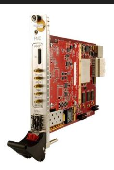
The pi827 is a COTS integration combining the flexibility of a Kintex-7 FPGA PXIe card (<u>PXIe/700</u>) and a 12bit 2.7GSPS ADC with 16-bit dual channel 2.8GSPS DAC (<u>DAQ2P5</u>).
